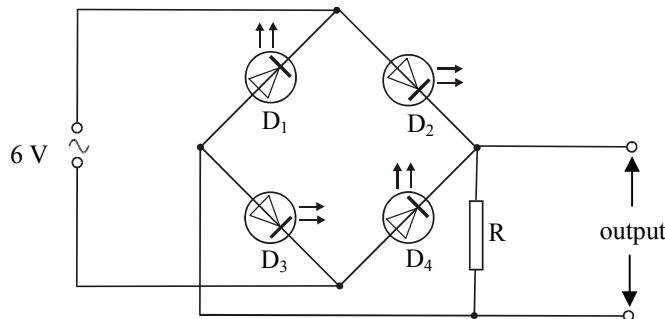
The circuit shows four light-emitting diodes connected to a resistor R and a 6 V a.c. supply of frequency 1 Hz.
